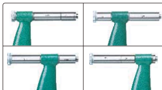
adjust collars for different measuring ranges
